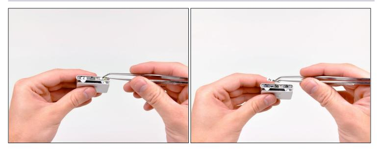
• Use a pair of <u>tweezers</u> to remove the hold and shuffle sliders from the Shuffle.
