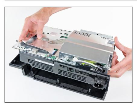
Lift the motherboard assembly out of the lower case.
