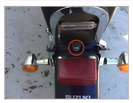
Remove the 4 mm Hex screw securing the back of the seat.
