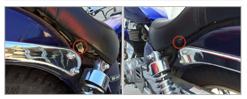
Remove the two 10 mm hex head bolts, one on either side of the seat.
