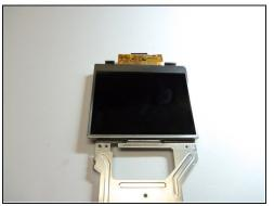
• Grab the end of the screen, then pull towards the inside of the case. This is a bit tricky. This will release tabs at the top of the screen to the rear case.
