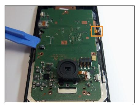
Pry the motherboard up using the plastic opening tool.
