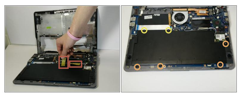
Remove the tape holding the wires in place.
