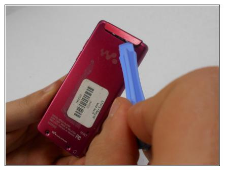
• Use a plastic opening tool to loosen the top panel of the device.
