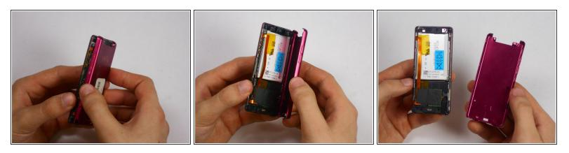
• Remove the back plate from the device.
