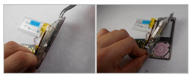
• Disconnect the metal shielding plate from the front panel with tweezers or a plastic opening tool.
