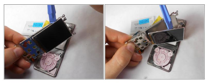
• Use a plastic opening tool to remove the screen from metal back plate.
