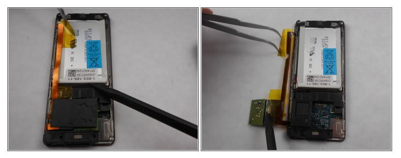
• Peel back the layer of tape along with the processor, which is located just below the battery, using the tweezers and the spudger.
