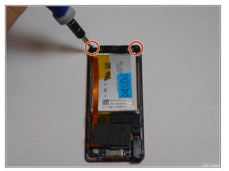
Use a Phillips #00 screwdriver to unscrew two 2 mm screws located on the top corners of the device.
