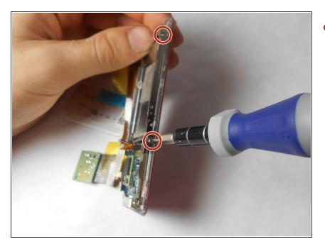
Use a Phillips #00 screwdriver to remove two 3 mm screws at the bottom sides and two 1 mm screws at top sides of the device.
