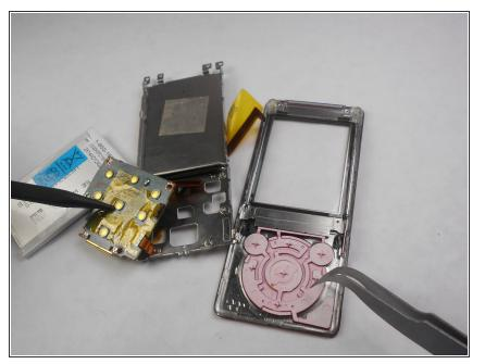
Ensure that button connection is completely separated from the buttons.
