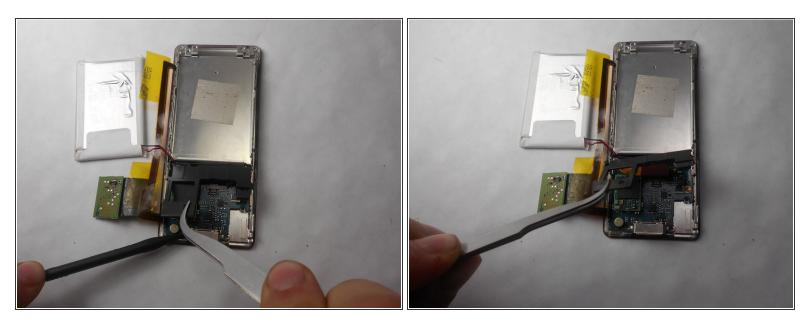
• Remove the plastic protective frame located over the motherboard with tweezers and a spudger.
