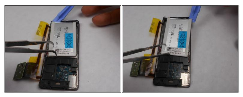
• Slide a prying tool underneath the top portion of the battery and lift it from the case.
