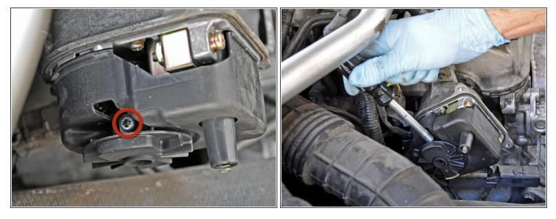
Remove the single #2 Phillips screw securing the distributor rotor to the shaft.
