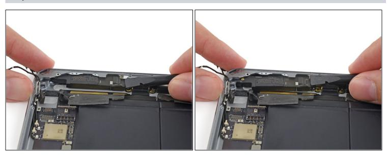
• Push the speaker with the flat end of a spudger to begin sliding it out of its recess in the rear case.
