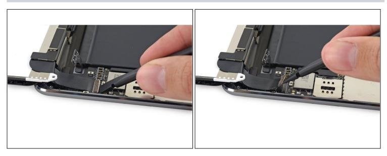
• Use spudger to lift the LCD connector up off its socket on the logic board.
