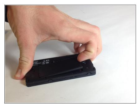
• To remove the battery, simply use your finger to pry the battery out of its slot.
