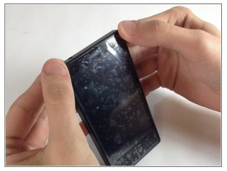
• The first step is to remove the back cover off of the phone. To do this, place both your thumbs on the two top corners of the device and simply pop it off.
