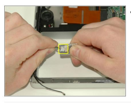
Disconnect the Bluetooth data cable from the Bluetooth board.
