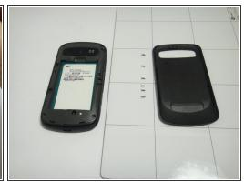
• Use the Phillips #00 Precision Screwdriver to remove the six screws in the back of the phone.
