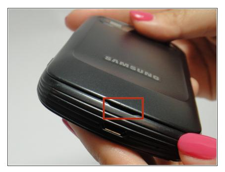
Use your fingernail or plastic opening tool to pull up the back cover of the phone from under the slit.
