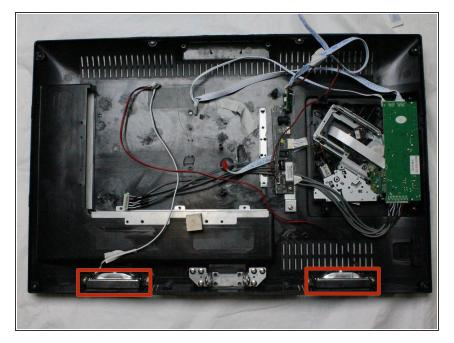
Locate the two speakers along the bottom of the plastic casing.
