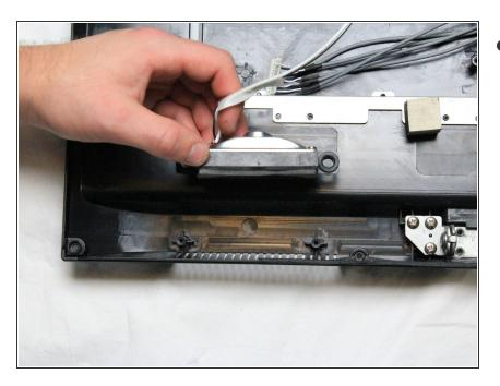
Lift up each speaker to remove it from the TV. The wires should already be unplugged from the motherboard and the speakers should now be completely isolated.
