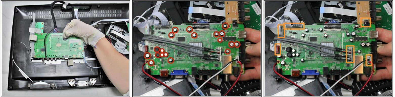
**⚠ Caution:** Before you remove the motherboard, be cautious of the many capacitors throughout that could cause serious injury or death. Use a discharge probe to safely rid the capacitors of dangerous charges. The following link provides an instructional video for how to properly complete this step: <https://www.youtube.com/watch?v=M-AlbrbT...>
