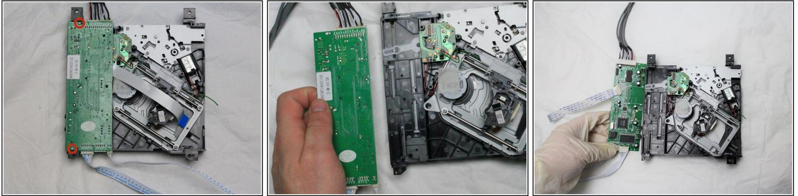
**⚠** This step involves working around capacitors. Before you remove the circuit board, be cautious of the many capacitors throughout that could cause serious injury or death. The following link provides an instructional video for how to properly complete this step:
