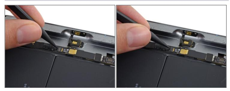
• Use the tip of a spudger to flip the microphone cable ZIF connector tab.
