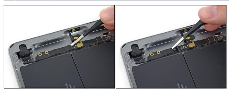
• Use a set of <u>tweezers</u> to peel back any tape covering the dual microphone cable connector.
