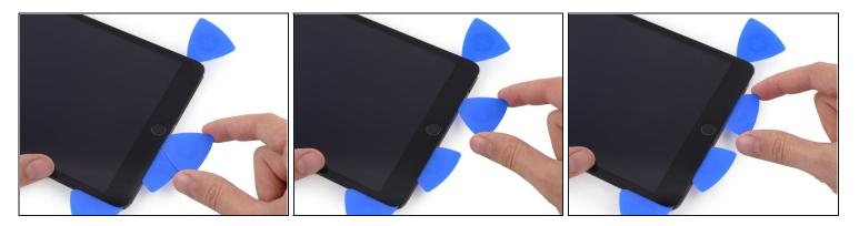
• Insert the tip of one last pick next to the previous step's pick, and slide it beneath the home button.
