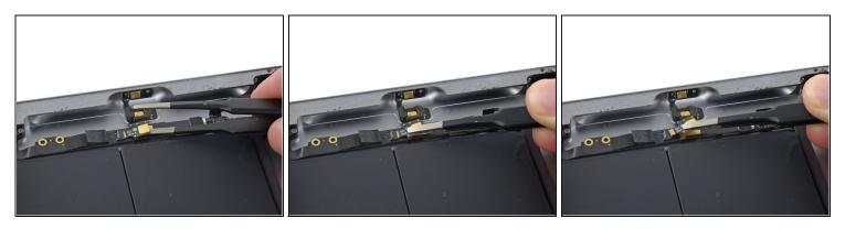
• Slide one end of a set of tweezers under the microphone cable and pull it out of its socket.
