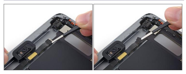
• Use a set of <u>tweezers</u> to remove any tape covering the front-facing camera cable clips.
