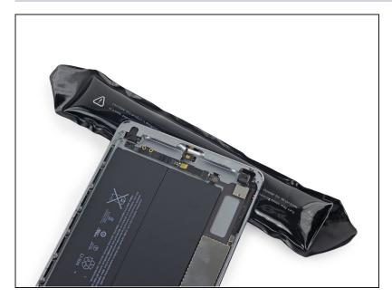
• Heat an iOpener and lay the iPad on it, to heat the microphone adhesive.
