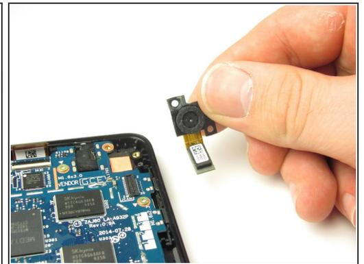
**⚠** Be careful not to damage the camera lens as you remove the camera.
