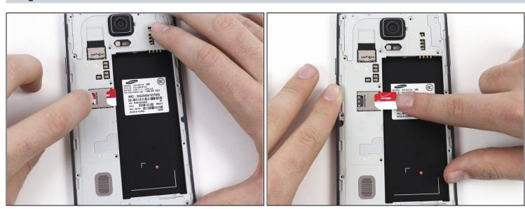
• Remove the SIM card by first pushing the card slightly out of its housing, then pulling it the rest of the way.
