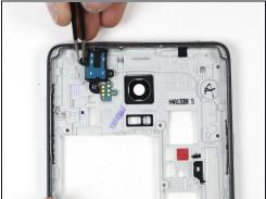
• Use the plastic spudger and <u>tweezers</u> to remove the headphone jack from the middle housing.
