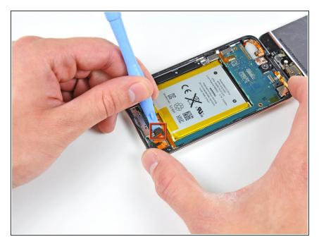
Use an iPod opening tool to pry the headphone jack connector up and out of its socket on the logic board.
