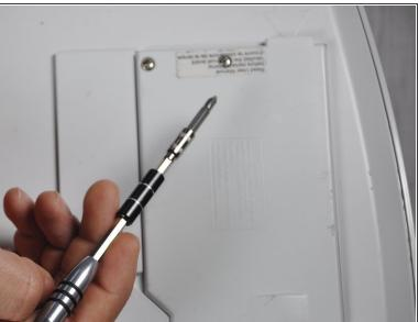
Use a Phillips #1 screwdriver to loosen the screws that secure the panel on the bottom of the Optoma HD20.
