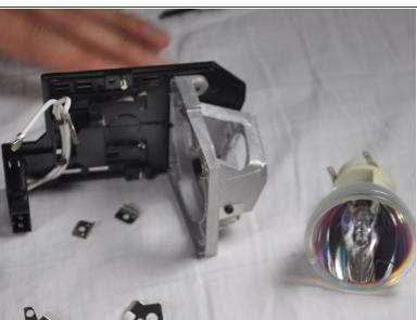
Remove the casing, then gently pull out the old light bulb and replace it with the new one.
