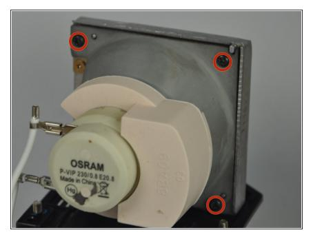
Remove the three 4.5 mm screws on the light bulb case.
