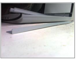
• 4. Then undo the three screws on the rail. You can lift out the metal rail. Place it on a flat surface to see if it is bowed, and if so, gently bend it flat.
