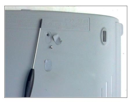
Firstly turn over the scanner and remove the 3 screws on the back of your scanner which are covered by plastic dark grey oval strips (2 at extremes, 1 in center; the 2 covers in between these can be ignored). This is so you don't have to turn the scanner over latter when parts may fall out. These screws hold the metal 'spine' in place.
