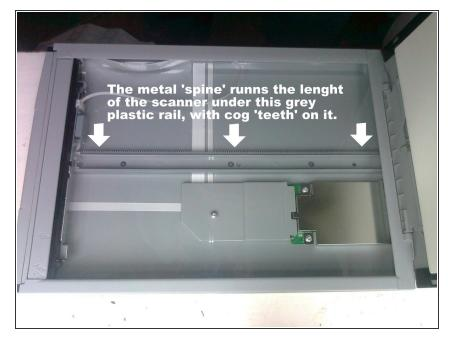
The metal 'spine' you are going to re-shape is under the grey plastic rail with the 'cog teeth' that you can see inside the scanner.
