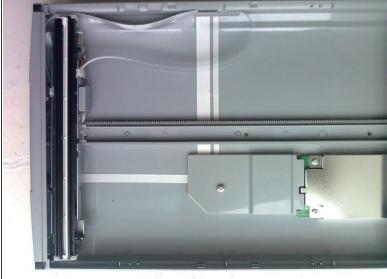
Now gently lift the scanner head off the grey plastic rail and place it to one side of the case out of the way.
