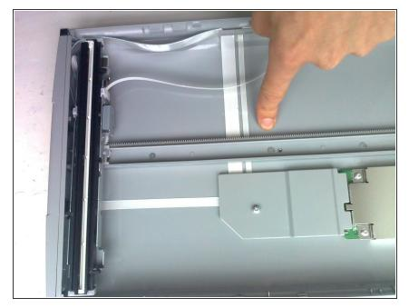
At this point you can test again to see if the scanner back is bowed by pressing the casing in the centre of the base with your fingers to see if it dips towards the table/surface it is on.
