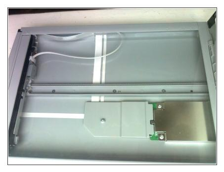
5. Now reassemble the entire scanner again. You can use double sided sticky tape to stick the plastic rail on again. I hope this helps you.
