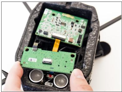
Carefully pull the secondary board from the mainboard.
