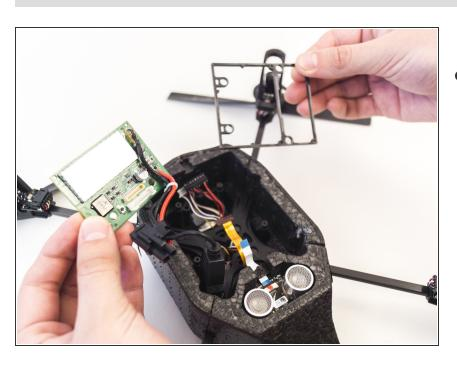
The mainboard is now fully detached and can be removed. To reassemble your device, follow these instructions in reverse order.
