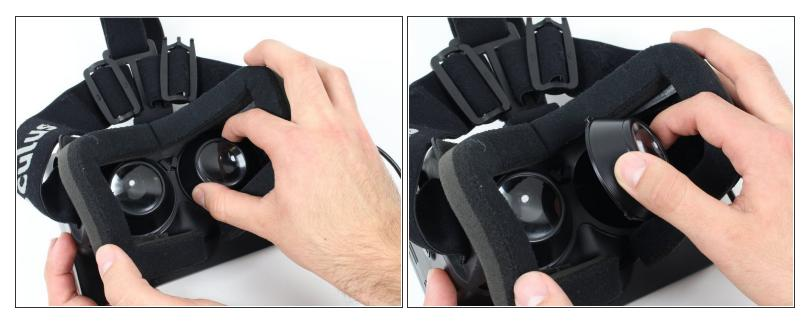
• To remove the lenses, turn the right lens clockwise a quarter turn and the left lens counterclockwise a quarter turn.
