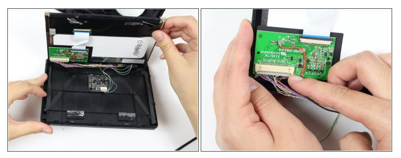
• Remove the wires from the circuit board on the LCD display using your fingernail or a plastic opening tool. This may take some pushing and pulling of the plastic piece.
