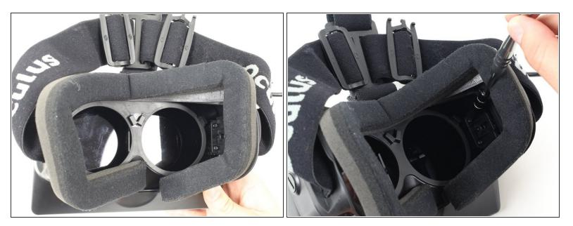
• Use a Phillips #01 screwdriver to unscrew the four 9 mm Phillips #01 screws. (Two screws are shown in the picture, and two more screws are on the left side across from the right screws.)
