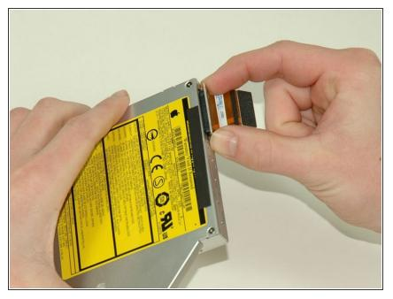
• Disconnect the orange ribbon cable from the back of the optical drive.
