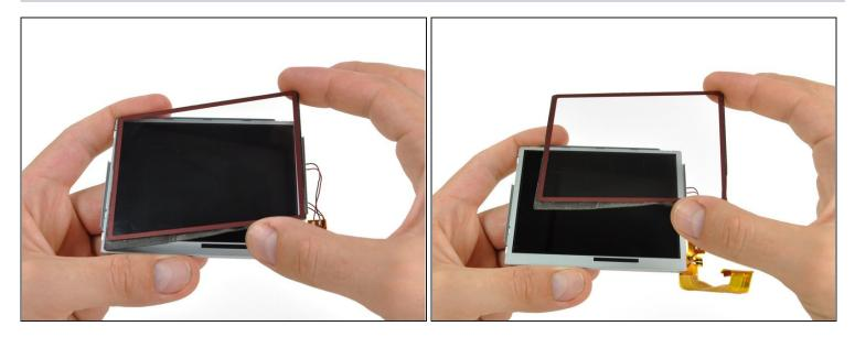
• Firmly grasp the upper screen, and lifting from the right edge, pull the upper screen off of the upper LCD.
