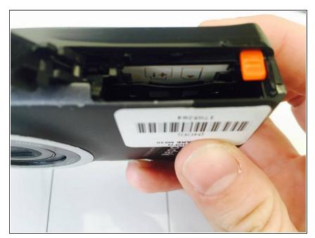
The diagram shows the (-) side should be on your right, while the (+) side should be on your left. Insert the new battery and memory card here.
