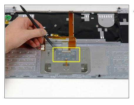
Use a spudger to pry up the translucent plastic sheath covering the keyboard connector.
