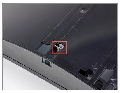
⚠ Be sure to keep track of the small metal bracket loosely held in the top cover, if equipped.
