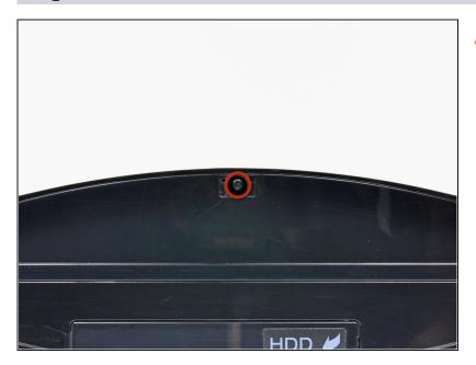
Remove the single 8.5 mm T10 Security Torx screw from the smart plate.
