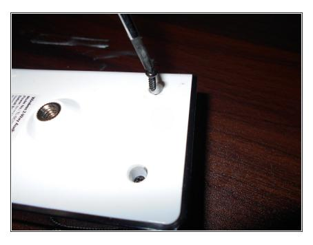
Remove the 2 screws holding the back cover!Should be fairly easy(You need a Phillips Screwdriver)
