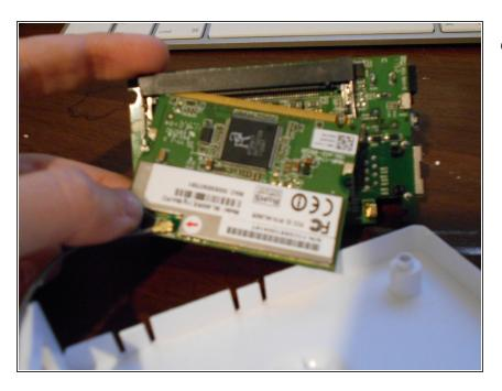
Remove the wireless card which is hold by 2 "clips"!
