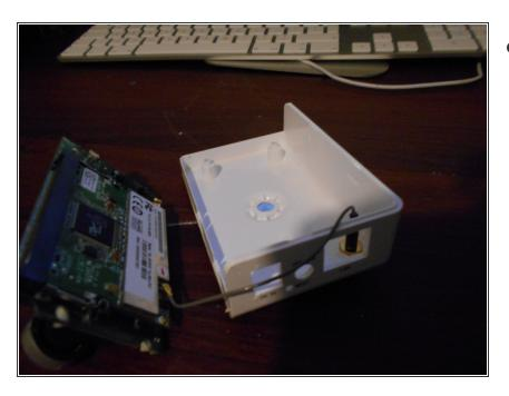
Remove the board from the Surveillance Camera!
