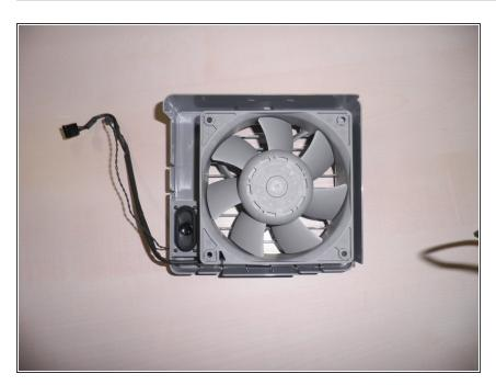
Left Fan in processor cage with speaker.
