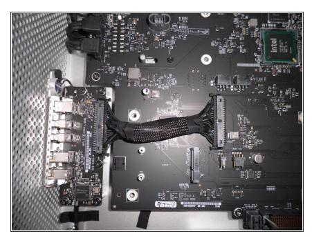
BackPlane Board and frontPanel Board linked by FrontPanel Board to BackPlane Board cable
