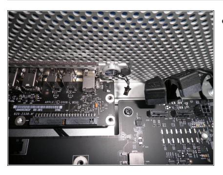
A view of the power button that needs to be connected on the front panel board.
