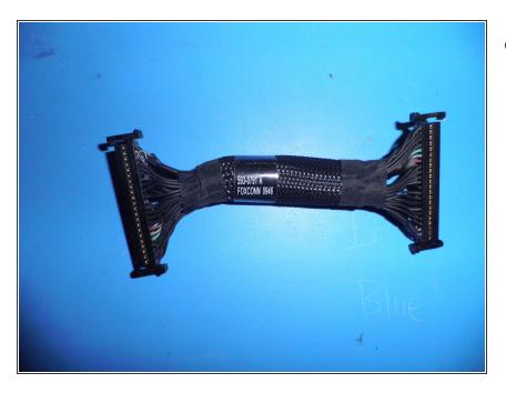
The front panel board to backplane board cable
