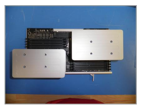
Processor heatsinks 8 Core
