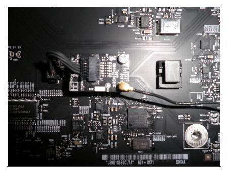
Bluetooth antenna connected to the card on the Backplane board. One needs to be careful because if not connected the Antenna needs to be attached in order not to short-circuit the backpanel board.
