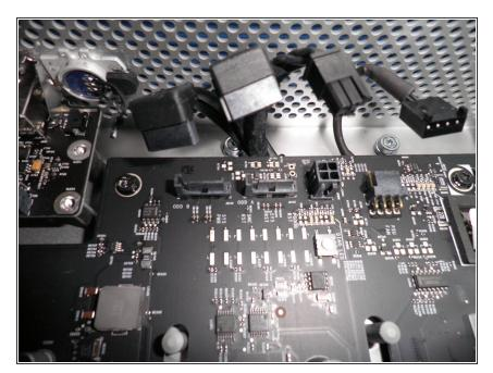
Optical Drive Cables on BackPlane Board.
