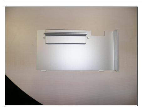
Small parts that cover the PSU and Super Drive cables.
