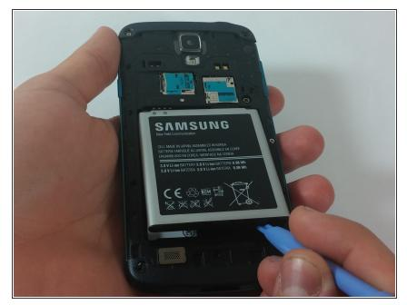
Insert a plastic opening tool, or your finger, into the notch of the battery compartment and lift the battery upward to remove it.
