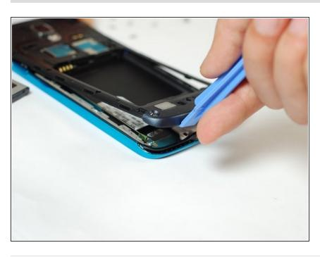
Use the plastic opening tool to pry around the entire edge of the midframe now to release it from the front case.
