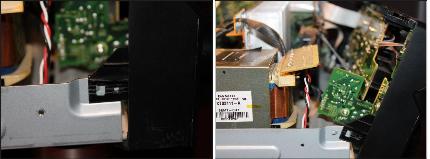
**⚠ Once the unit is reassembled, these zipties must be replaced. Failure to do this will result in protection mode errors.**
