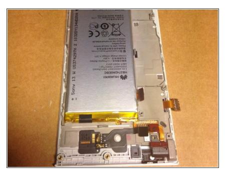
The battery is held down with two small pieces of double-sided tape.
