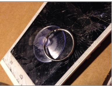
If your display is badly cracked, it is recommended to apply tape to keep the shards of glass contained. It will also help using a suction cup later on in the process.
