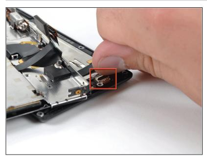
• Remove the front panel ribbon cable from the ZIF connector on the board that is attached to the display ribbon.
