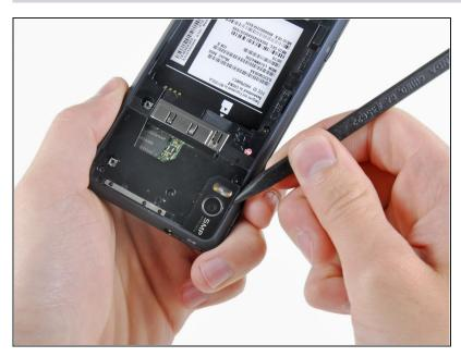
Use the tip of a spudger to remove the camera bezel stuck to the rear case.
