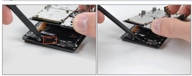
• Use the tip of a spudger to lift the speaker out of the screen housing.
