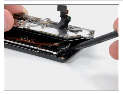
Use the flat end of a spudger to lift the board that contains the ambient light sensor and display data cable connector out of the screen housing.
