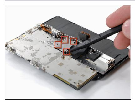
Remove the EMI shield by releasing the clips shown with the tip of a spudger.
