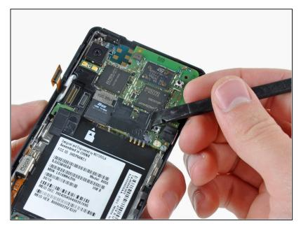
Use the flat end of a spudger to remove the small black plastic piece stuck to the battery connector.
