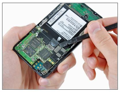
Disconnect the power button/volume button connector from its socket on the motherboard using the flat end of a spudger.
