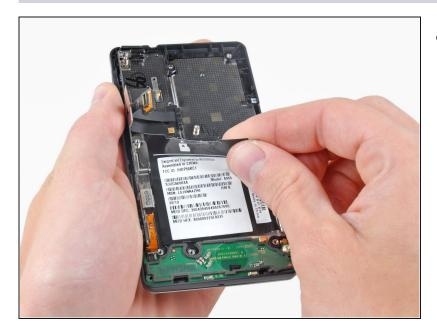
Remove the large sticker stuck to the inner face of the battery compartment.
