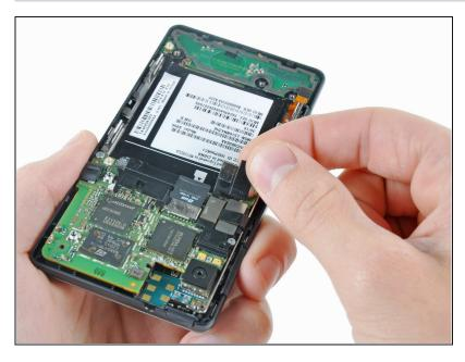
Peel the black rubber sheet covering the side button and display ribbon connectors on the motherboard.
