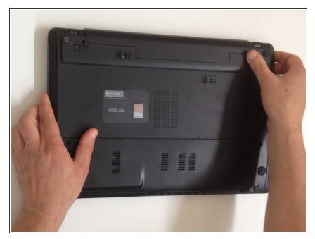
Switch off the laptop and remove the battery.
