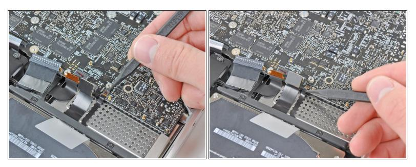
Use the tip of a spudger or your fingernail to flip up the retaining flap on the battery indicator cable socket.
