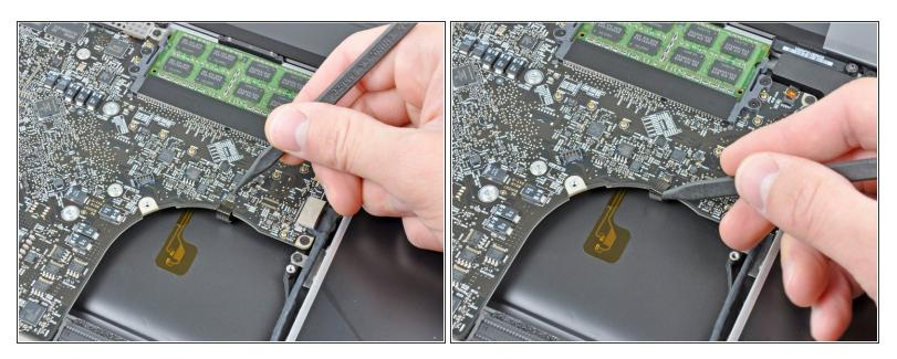
• Use the tip of a spudger or your fingernail to flip up the retaining flap on the keyboard backlight ribbon cable.
