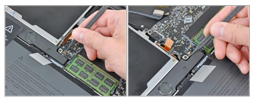
Use the tip of a spudger or your fingernail to flip up the retaining flap on the IR sensor ribbon cable socket.
