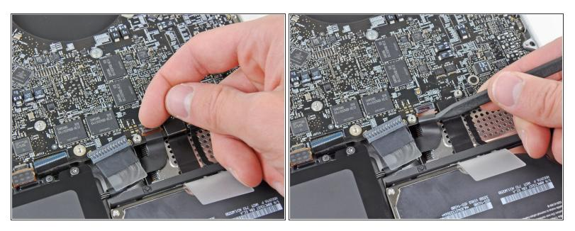
• Use your fingernail to flip up the retaining flap on the express card cage ribbon cable socket.
