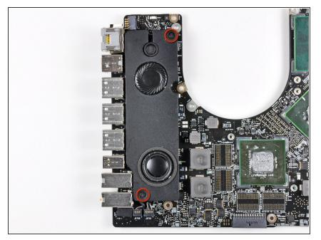
Remove the two 7.9 mm Phillips screws securing the left speaker to the logic board.
