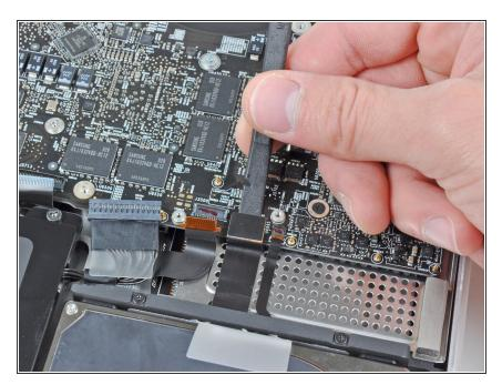
Use the flat end of a spudger to lift the hard drive cable connector up and out of its socket on the logic board.
