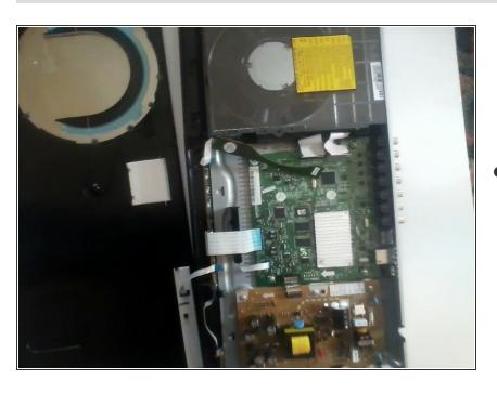
There is one screw holding the case on, and it is on the middle of the top of the back of the player. (Right above the outputs) IMPORTANT: When you take the case off, take especial care to not break any connections between the internal circuitry and the inside of the top casing. Fold it over like shown in the image.
