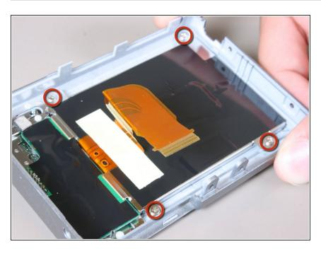
Using a #00 screwdriver, remove the four screws located at each corner of the LCD screen.
