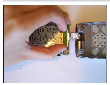
Pry the connector with finger nails.
