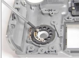
Remove two Phillips #00 screws from the inside of the button pad on the back cover.
