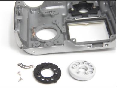
Remove the black ring from the back and the white button pad will fall out from the front.
