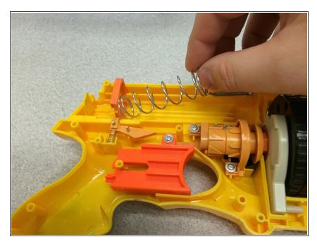
• Remove the larger spring from the catch mechanism.
