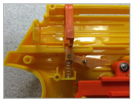
Carefully replace the catch mechanism so that it is seated in the grooves and over the metal pin.
