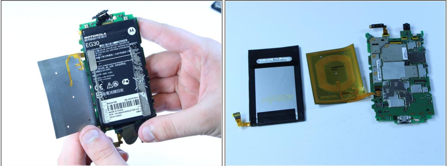
**⚠** Carefully peel back the orange adhesive from the battery. Make sure to remove all the adhesive attaching the battery to the motherboard.
