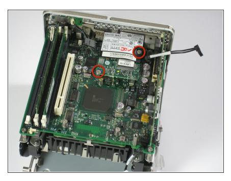
Remove the two screws from the modem.
