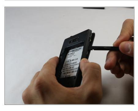
With the spudger, go around the seam of the phone and pry away the back chassis.
