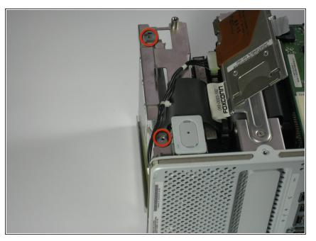
• Remove a total of four screws on the sides of the optical drive.
