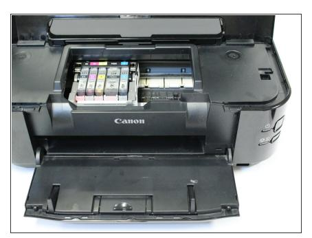
Allow the belt, containing ink cartridges, to adjust and center so that the ink cartridges are visible.
