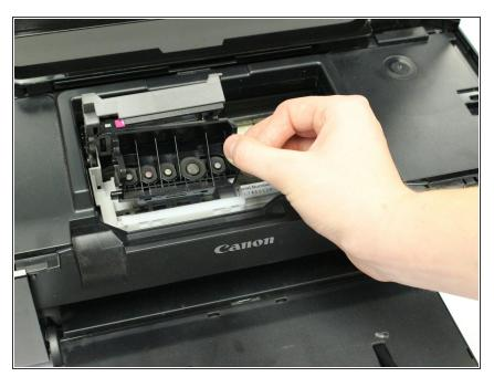
• Pull up and lift out the black piece that previously held the ink cartridges. This is the printhead.
