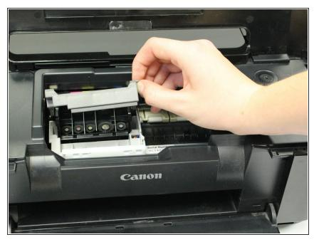
• After removing all ink cartridges, lift the printhead lock lever.
