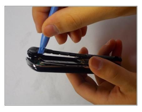
Insert the plastic opening tool in between the two halves of the case.
