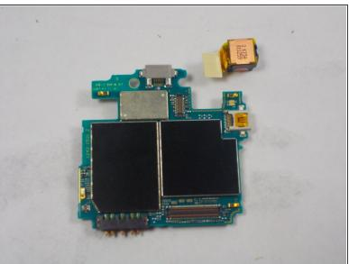
Lift the camera off of its connector on the logic board.
