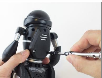
Remove the three 12.0 mm Phillips # 2 screws from the battery cover.
