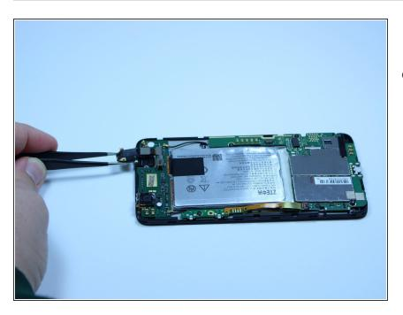
Using a pair of tweezers, gently remove the earphone outlet from its slot
