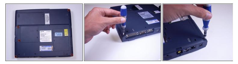
• Using a Phillips screwdriver, unscrew and remove 5 B20 screws, located along the corners of the bottom of the laptop.
