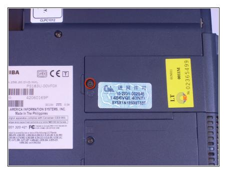
Using a Phillips screwdriver, unscrew and remove F4 screw from plastic covering on the bottom of the laptop that only has one screw.
