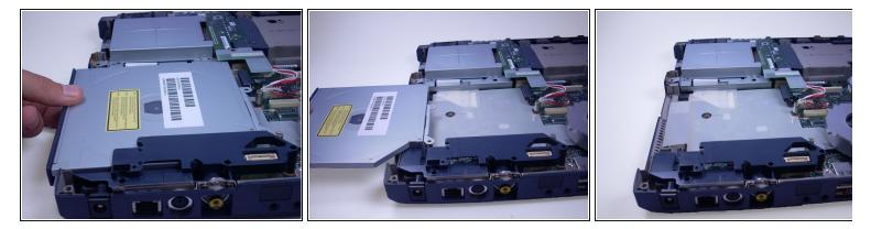
• Using your fingers, slowly slide the optical drive out of the laptop, towards you, until you are able to completely lift it away from the computer.
