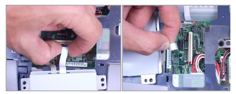
• Remove the white ribbon on the right by pinching the part connected to the laptop with your fingers and pulling towards you.
