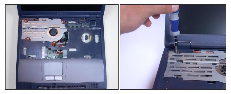
Using a Phillips screwdriver, unscrew and remove 5 screws labeled F6, located on the metal piece on the left side of the keyboard area.
