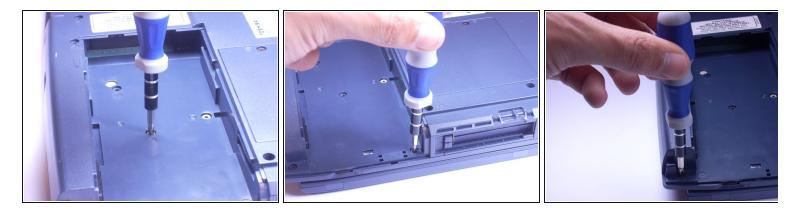
Using a Phillips screwdriver, unscrew and remove 3 F4 screws from the battery area of the laptop.
