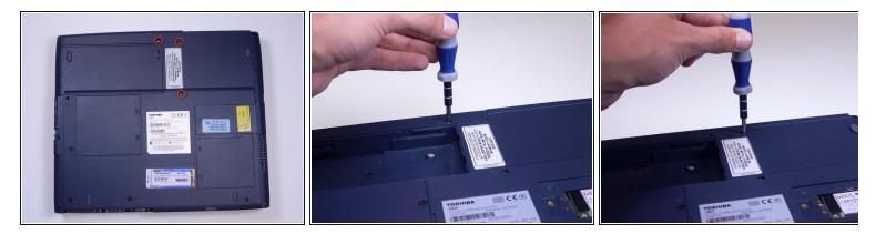
• Using a Phillips screwdriver, unscrew and remove 3 B25 screws from the bottom of the laptop.
