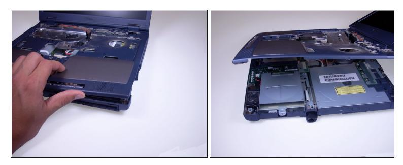
• Lift open the screen of the laptop and, using your fingers and the guides on the side of the laptop, push up on the top plastic covering of the laptop, moving from one side of the laptop to the other.
