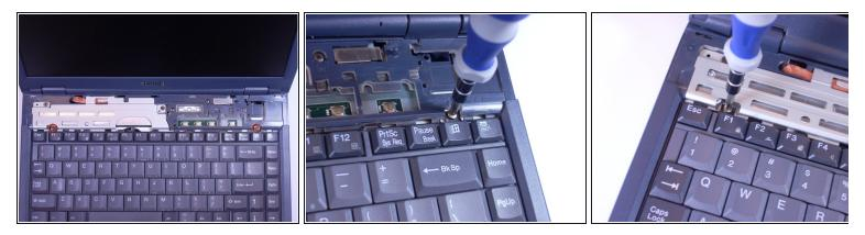
Using an Phillips screwdriver, unscrew and remove two screws labeled B2.6.
