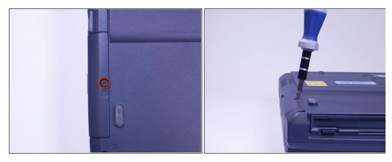
• Look at the bottom of the laptop. Using a Phillips screwdriver, unscrew and remove the screw labeled F4, located on the cover of the hard drive.
