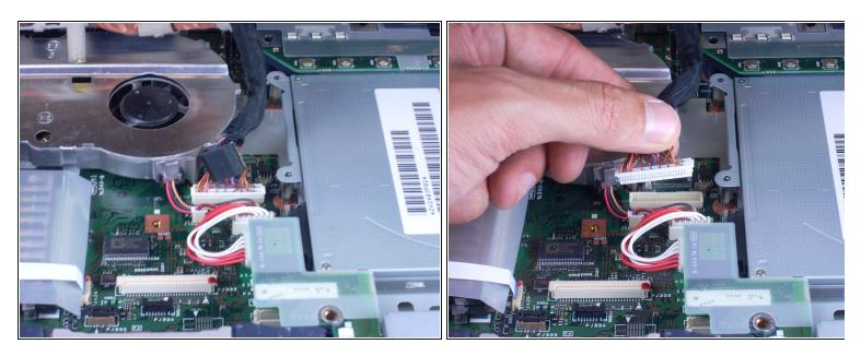
Setting screen next to the base of the laptop, pinch the connecting cable with your fingers and gently pull connecting cable from monitor.
