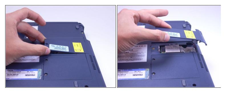
• Using fingers, pinch and lift plastic covering up, away from the laptop and set aside.
