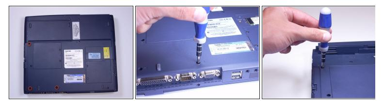
• Using a Phillips screwdriver, unscrew and remove 3 F6 screws from the bottom of the laptop.
