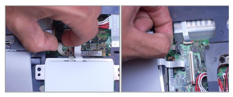
Remove the left, brown ribbon by pinching the part of the ribbon connected to the computer and lifting towards you.
