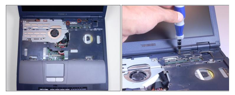
Using a Phillips screwdriver, unscrew and remove two screws labeled B25 located closest to the screen.
