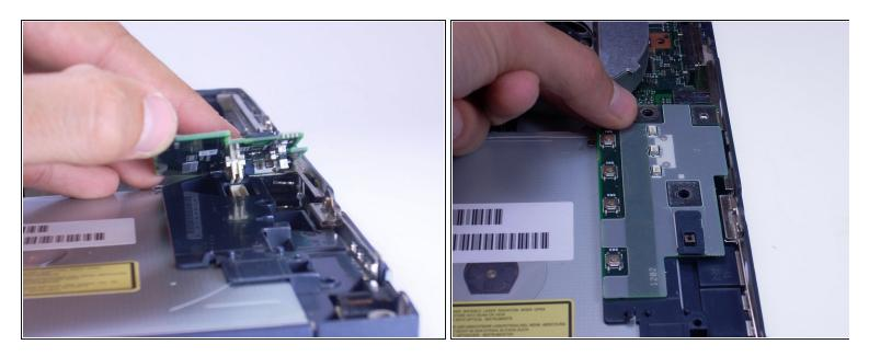
• As shown by the photo, remove the small green computer part by pinching the top with your fingers and gently lift it away from the laptop.
