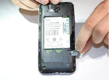
Remove the battery and SD card from the phone.
