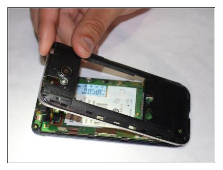
Remove the back piece, exposing the motherboard.
