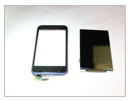
Dispose of the old font panel and replace it with the new one.
