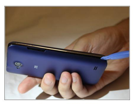
Using a spudger, remove the back panel of the phone.
