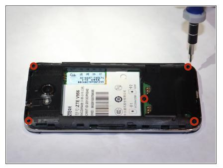
Remove the five 4mm Philips #00 screws, circled in red, holding the the back down.
