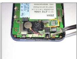
Flip up the three small tan clips holding the ribbons in place.
